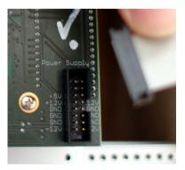
Jomox ModBase09/ModBrane11 euro rack supply connector. Please connect the power supply of the eurorack system bus *here*.
