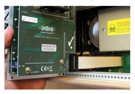
Then please mount the module on the rack rails with the supplied metric M3 screws. In case you want to connect a midi cable, please do this beforehand of mounting.
