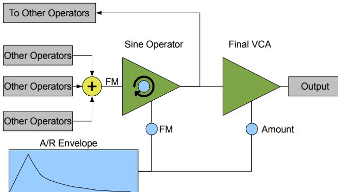
A sine operator is modulated by the outputs of the other 3 sine operators and can feedback its own output to the other FM operators. A simple Attack/Release envelope generator can FM-modulate the sine operator as well.
