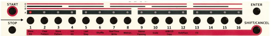
If the EDIT/TRIG LED is off, the **(Step)** buttons serve for selecting 16 patterns in a bank.
