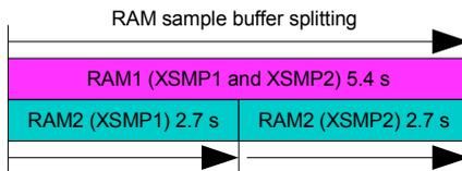
This also implies that, for instance, X1 may be set to RAM1 and plays the RAM buffer at full length, while X2 is set to RAM2 and starts at the second half of the RAM buffer.
