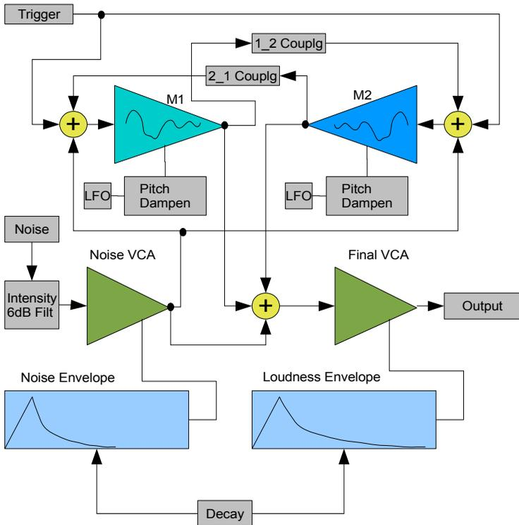
The sound production in the MBrane is made up of 2 filter oscillators (M1 and M2) that have the same frequency range of 25Hz - 14kHz.
