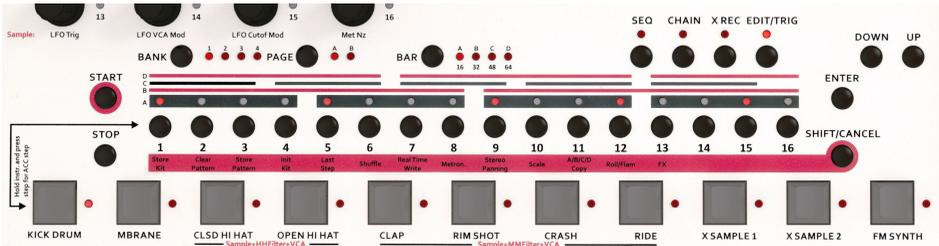
Press **(EDIT/TRIG)** so that the LED is on then select a track by pressing an instrument key. Press **(Start)** to let the sequencer play.
