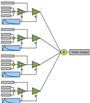
Up to 6 voices can be played. The 6 voices can be addressed by an external midi keyboard which plays them polyphonically. The chord is stored in the preset and is played as a fixed chord by the internal sequencer according to the maximum number of voices. This chord is shifted in whole by the sequence play function SEQ.
