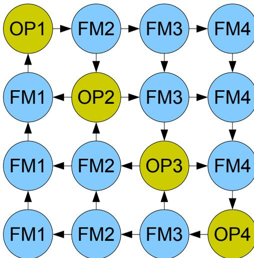
Each knob of the green diagonal is one operator and the knobs OP1-OP4 control the base frequency of that operator.
