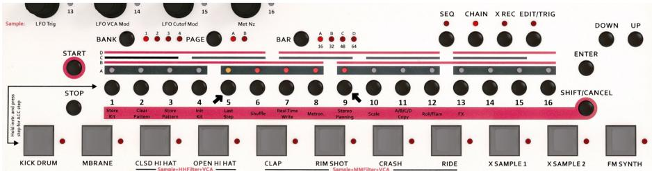
All step LEDs between the both steps light up and the selected patterns are played in a chain from left to right, beginning with the leftmost and cycling back after having played the last one. The currently played pattern blinks orange. The chain information is stored along with the first pattern of the chain. Don't forget to store the pattern with Pattern Quick Store (**Knob 15 click**) or Store Pattern (**Shift 3**).
