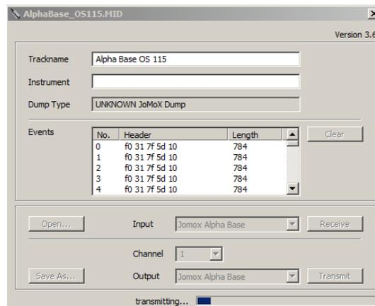
4. Now just press Transmit. You don't need to adjust anything on the Alpha Base. The blocks start to count up in the Alpha Base display while the progressing bar on the tool grows.
