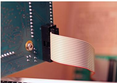
Connect the other end of the ribbon cable to the module as shown on the picture. The cables are fairly short which is good in electrical regards to the relatively high power consumption of the module.
