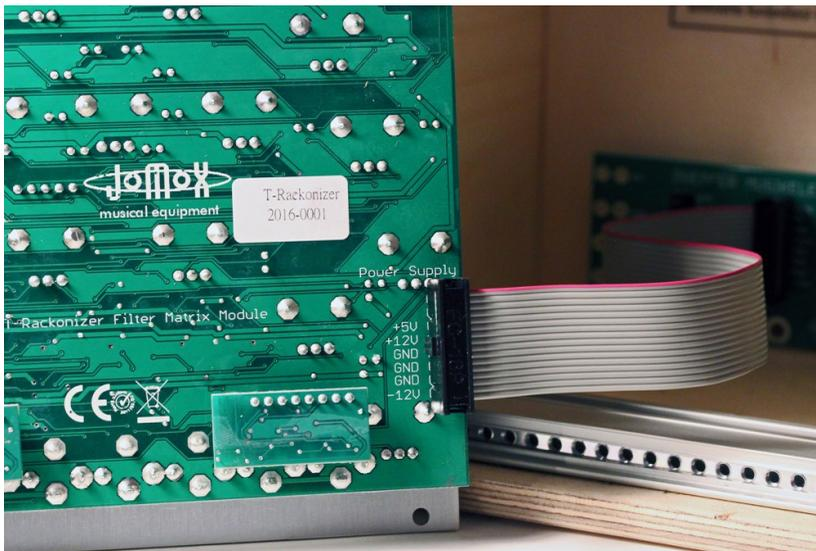
**Attention: DO NOT connect, under any circumstances, the power supply cable to the Jomox Inter-D-module bus!!! The rack power supply and the module could get seriously damaged!**
