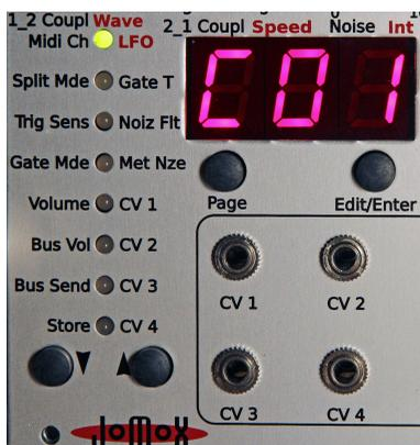
The Mod.Brane 11 has an up/down menu with 8 rows and 3 pages which are shown by multi-colored LEDs.
